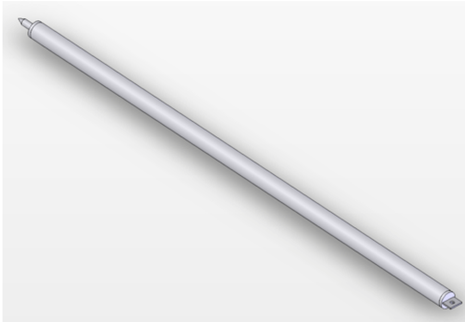
Figure C-10: Lightning Protector Rod
