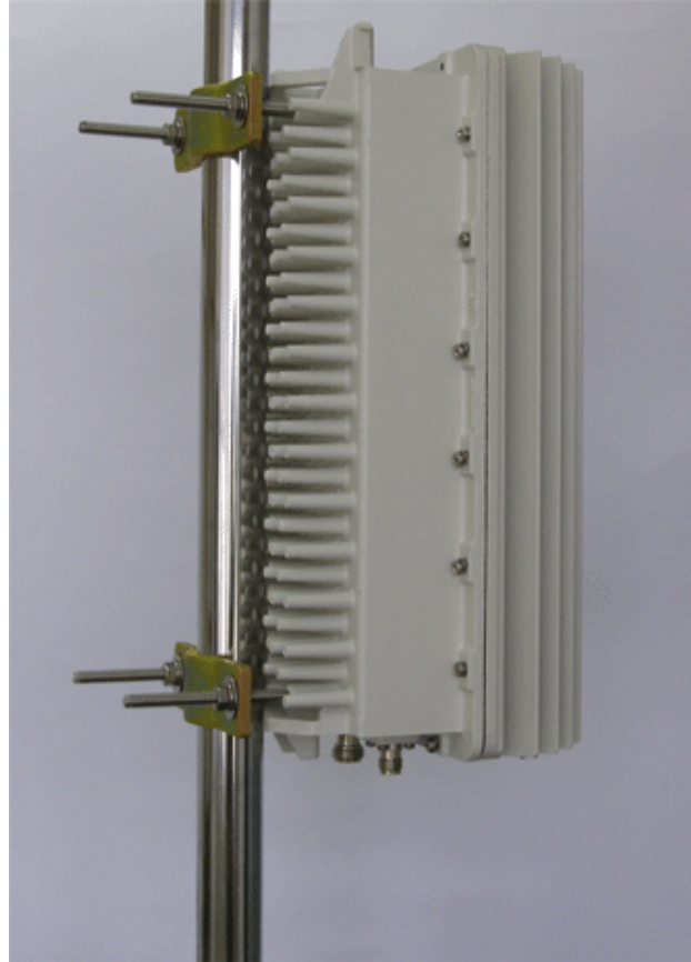
Figure 5-24: AU-ODU-HP Assembled on a Pole
